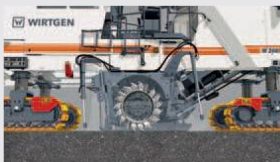
2 | The milling machine is lowered quickly while retaining its parallel alignment
