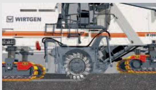
4 | The milling machine mills at full working depth right from the first metre
